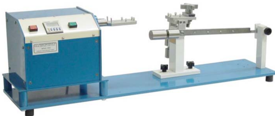
FIG. 1 Device for Preparing Twisted Pair Specimens, Motorized Unit
