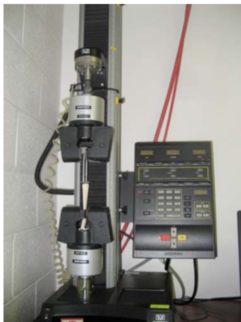
FIG. 3 Tensile Test Machine and Clamped Test Specimen
