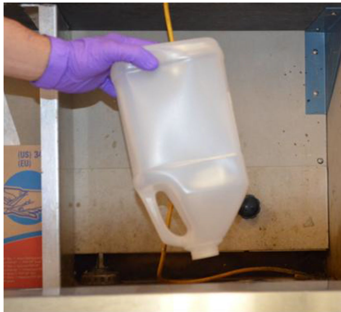
FIG. 1 Draining of Sample Container with a Spout
