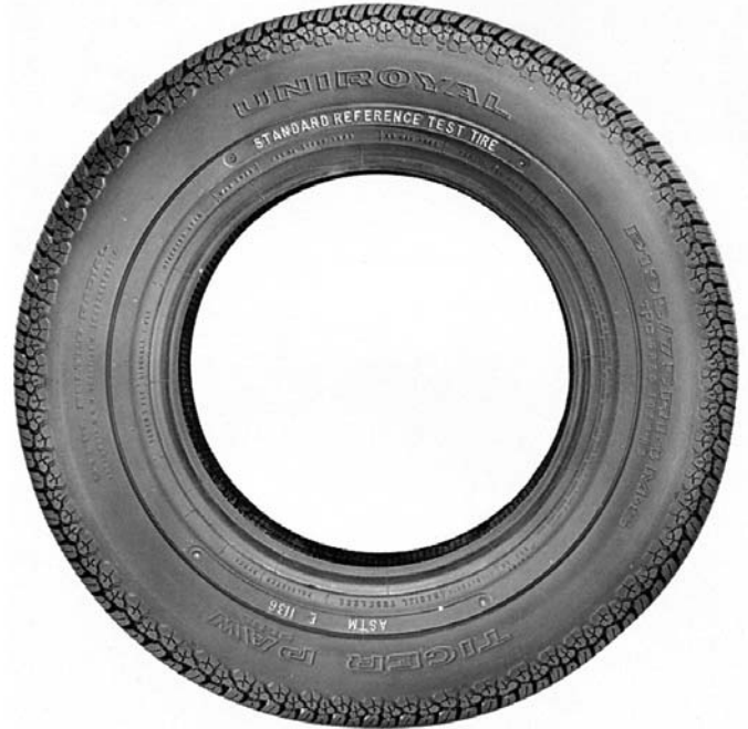
FIG. 2 Side View of the P195/75R14 Radial Standard Reference Test Tire
