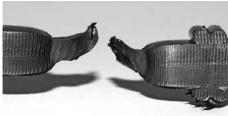
FIG. 2 Ductile Rupture Outside Fusion Interface
