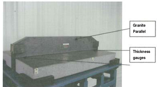
FIG. 4 Example of a Table and Granite Parallel Used to Measure Straightness by the Roll Test
