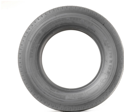
FIG. 2 Side View of the 245/70R19.5 136/134M Radial Truck Standard Reference Test Tire
