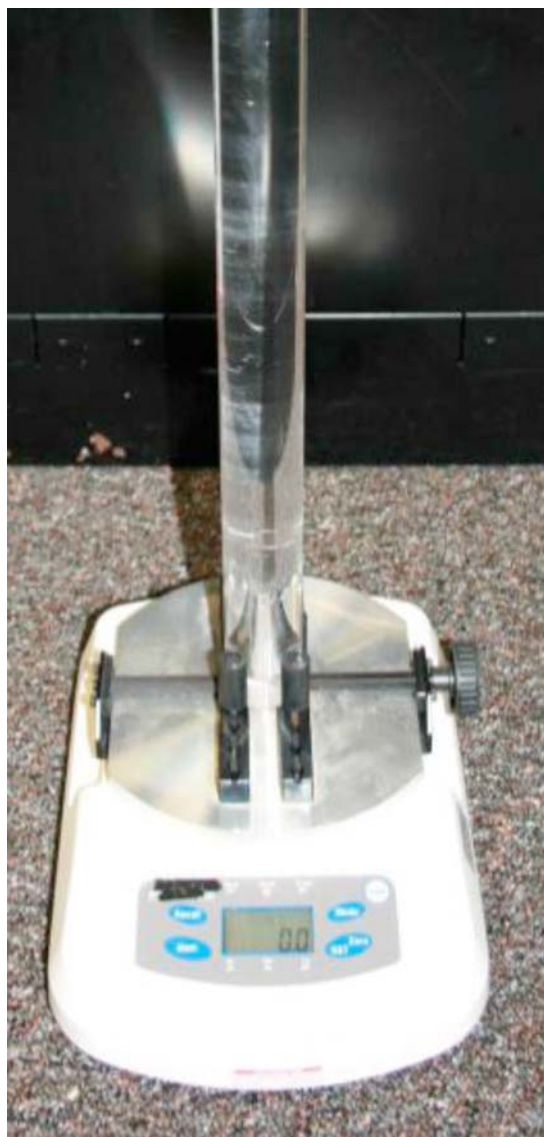
FIG. 1 Acrylic Rod Attached to a Torque Meter
