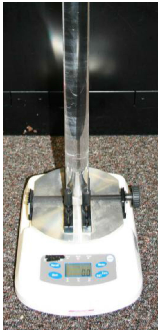
FIG. 1 Acrylic Rod Attached to a Torque Meter
