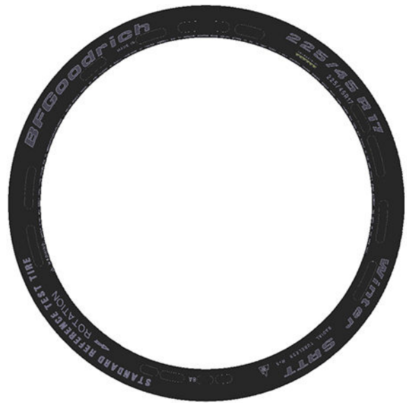
FIG. 2 Side View of the 225/45R17 94H XL Radial Standard Reference Test Tire
