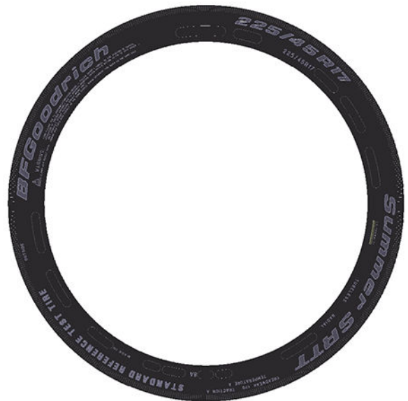
FIG. 2 Side View of the 225/45R17 94V XL Radial Standard Reference Test Tire
